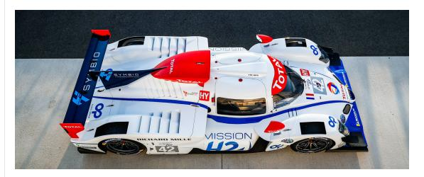
Externally, its bodywork, still developed by the Addess Company, marks a complete rupture with that of the previous model. Its shape reflects the gains obtained: improved aerodynamic performance and better cooling for the propulsion system.
